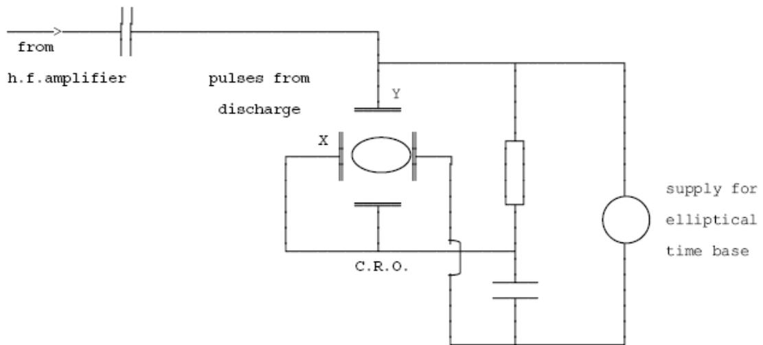
The oscilloscope X and Y plates are supplied from a separate source so as to form an ellipse on the screen. By applying the output from the high frequency amplifier to the Y-plates, we can obtain the high frequency pulse superposed on the ellipse. The height of the pulse can be measured.
