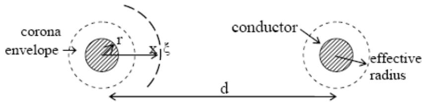
The electric stress  $\xi$  at a distance  $x$  from a conductor of radius  $r$ , and separated from the return conductor by a distance  $d$  is given by,
