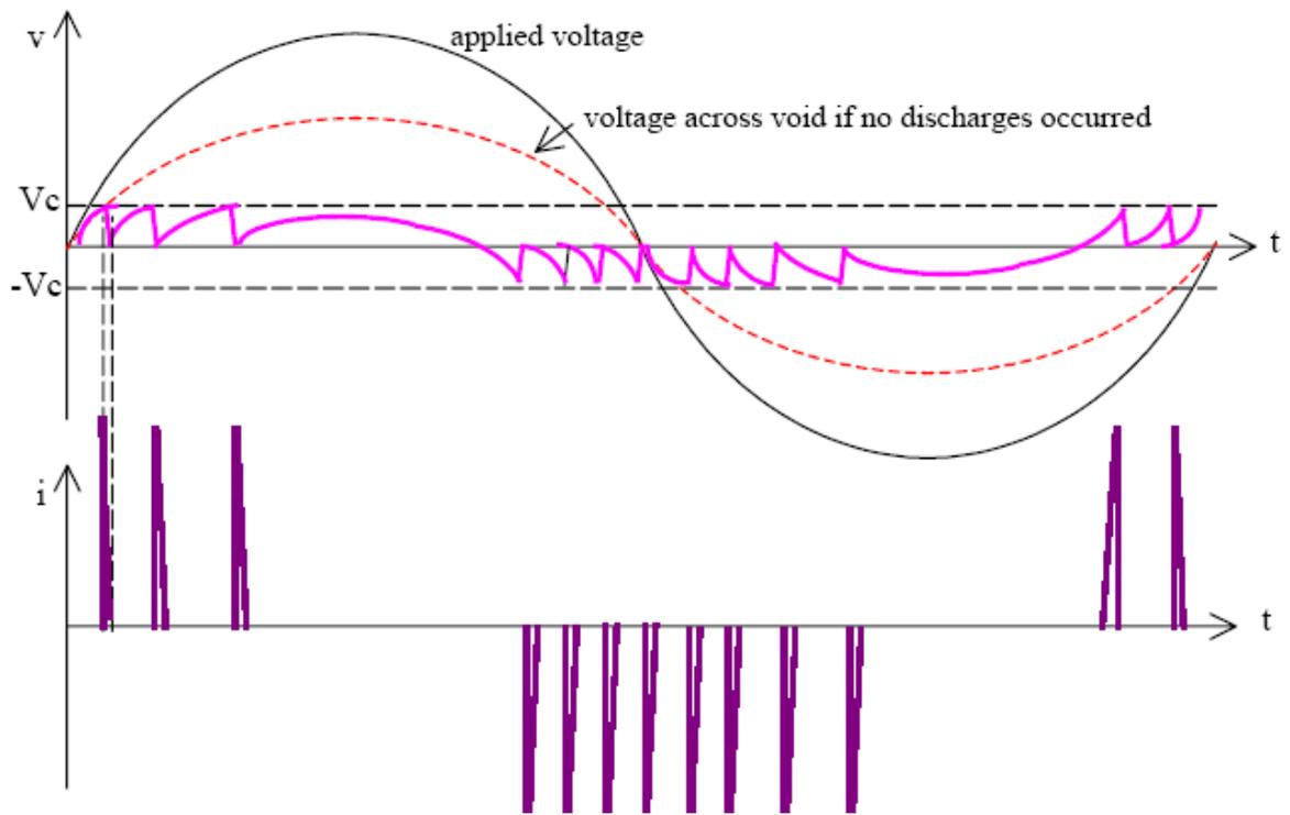
In each of the discharges, there will be heat dissipated in the voids which will cause carbonization of the surface of the voids and erosion of the material. The gradual erosion of the material and consequent reduction in the thickness of the insulating material eventually leads to breakdown. Breakdown by this process is slow and may occur in a few days or may take a few years.
