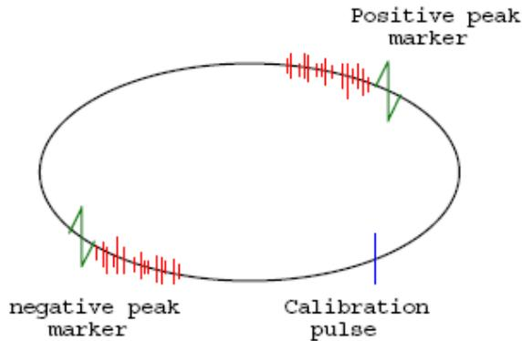
The above figure shows a typical oil-impregnated paper capacitor: The discharges are approximately equal in magnitude and numbers in the two half cycles, but have opposite polarity.
