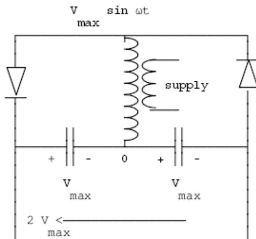
In this case, the transformer will be of small rating that for the same direct voltage rating with only simple rectification. Further for the same direct voltage output the peak inverse voltage of the diodes will be halved.
