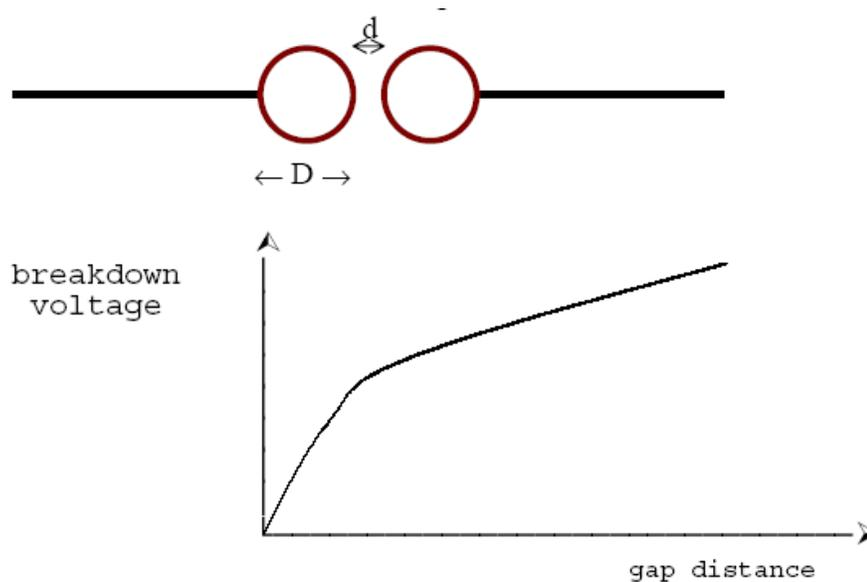
When the gap distance is increased, the uniform field between the spheres becomes distorted, and accuracy falls. The limits of accuracy are dependent on the ratio of the spacing  $d$  to the sphere diameter  $D$ , as follows.
