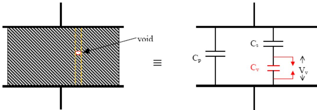
When the voltage  $V_v$  across the void exceeds the critical voltage  $V_c$ , a discharge is initiated and the voltage collapses. The discharge extinguishes very rapidly (say 0.1  $\mu$ s). The voltage across the void again builds up and the discharges recur. The number and frequency of the discharges will depend on the applied voltage. The voltage and current waveforms (exaggerated for clarity) are shown in figure below,
