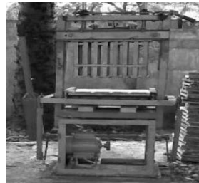
Figure 2, Interlocking block casting Machine
