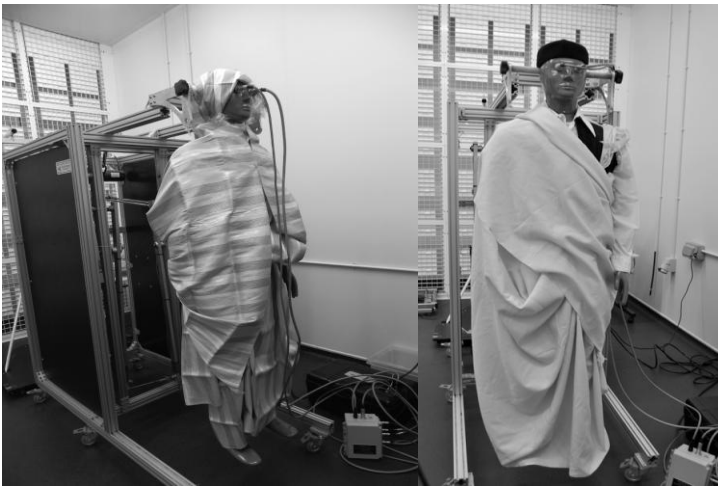
Figure. 4, the traditional Libyan clothing for female and male worn on the thermal manikin (Newton)
