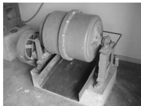
Figure 4, Ball mill to grind the burnt husk
