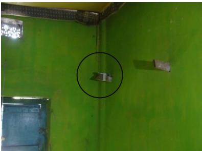
Figure 15, Installed Data Logger in Brick house
